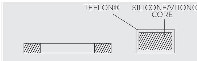
The seamless, uniform and integral TEFLON® encapsulation of the O-Ring is responsible for the sealing effect, whereas the continuous reset and the constant pressure of the encapsulation onto the sealing point is accomplished by the elastomer core. The result is an overall sealing compression, increasing with medium pressure. The encapsulated O-Ring behaves like a highly viscous fluid, any pressure exerted on the seal is transmitted practically undiminished in all directions.
