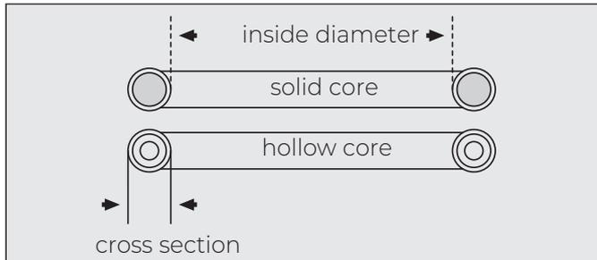
The encapsulated seal can also be supplied in a rectangular section. For these profiles the section diameter must not be less than 2.62mm to provide sufficient elasticity. See also Hose Coupling gaskets.
