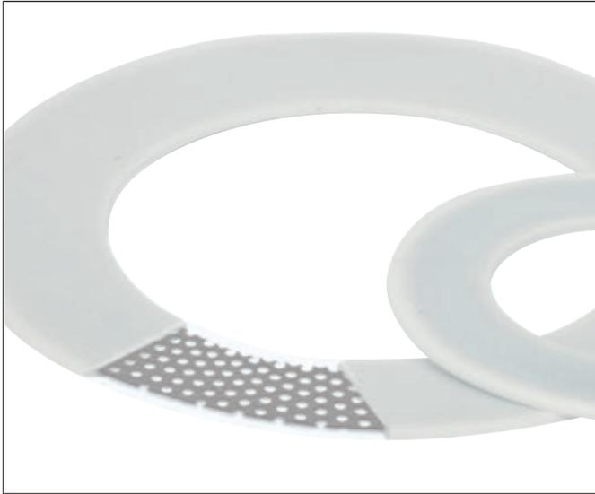
This is a flange gasket consisting of a 304 stainless steel wire mesh insert, individually moulded into a virgin P.T.F.E. ring conforming to ASA and DIN standards. It is ideally suited for use in a corrosive environment and its non-ageing qualities also make it perfect for use on joints which are not protected from the atmosphere.
