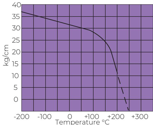
The recommended working pressure of a TEFMET gasket is dependent on the service temperature, and the stated values should be adjusted accordingly.
